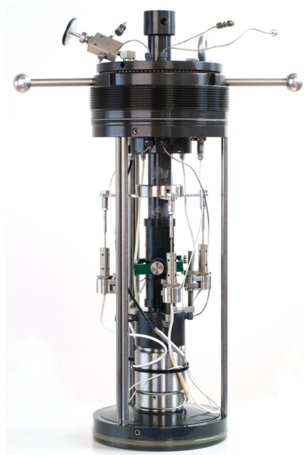
Set-up for a triaxial test including in-vessel load cell, three axial displacement transducers and one diametral extensometer.
