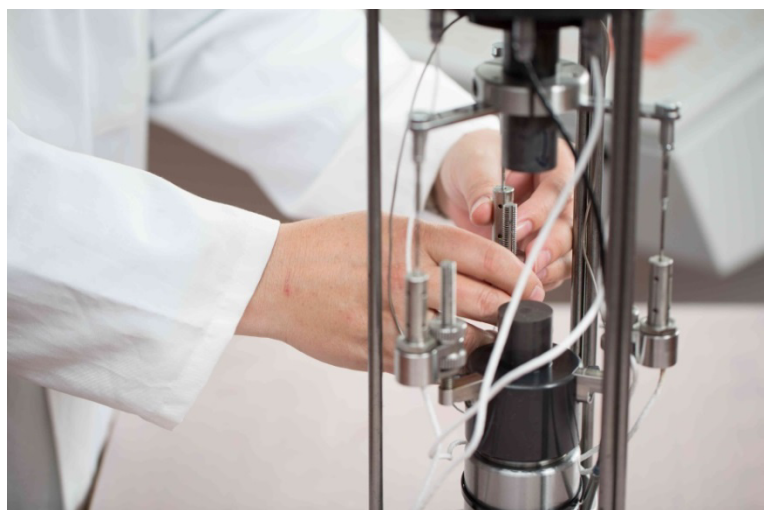
A LVDT-clamping device is mounted into a triaxial pressure cell. The device is equipped with an integrated fine-adjustment for up to three displacement transducers in a distance of 120° to each other
